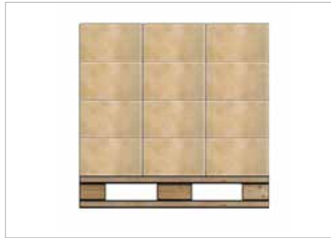
Fully covered and aligned
