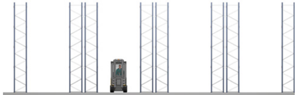
The most common conventional system comprises a single-entry rack fitted to the wall and double-entry racks in the middle
