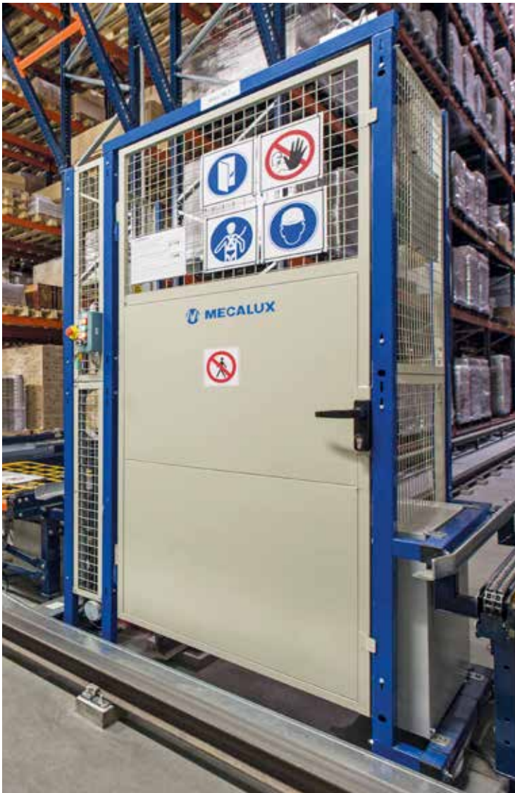
Control and maintenance zone partitions
